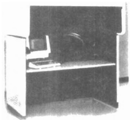
Figure 2-18 The SpaceGraph interactive graphics system displays objects in three dimensions using a vibrating, flexible mirror. (Courtesy of Genisco Computers Corporation.)
