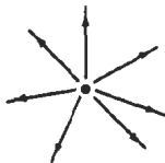
Figure 14-2 Diverging ray paths from a point light source.
