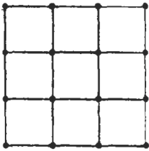
Figure 14-70 Subdividing a pixel into nine subpixels with one ray at each subpixel corner.
