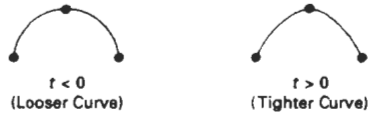
Figure 10-31 Effect of the tension parameter on the shape of a cardinal spline section.
