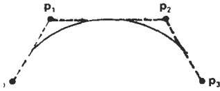
Figure 10-43 Quadratic, periodic B-spline fitted to four control points in the xy plane.
