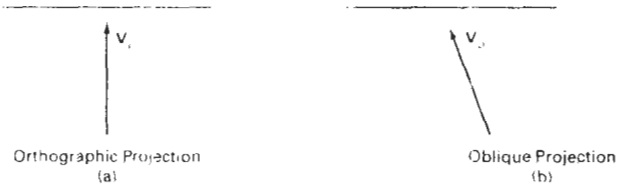
Figure 12-17 Orientation of the projection vector V_p to produce an orthographic projection (a) and an oblique projection (b).
