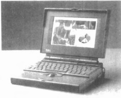
Figure 2-15 A backlit, passive-matrix, liquid-crystal display in a laptop computer, featuring 256 colors, a screen resolution of 640 by 400, and a screen diagonal of 9 inches. (Courtesy of Apple Computer, Inc.)
