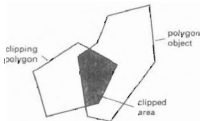
Figure 6-26 Clipping a polygon by determining the intersection of two polygon areas.
