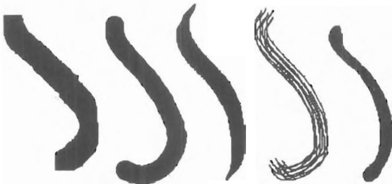
Figure 4-10 Curved lines drawn with a paint program using various shapes and patterns. From left to right, the brush shapes are square, round, diagonal line, dot pattern, and faded airbrush.
