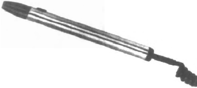
Figure 2-56 A light pen activated with a button switch. (Courtesy of Interactive Computer Products.)
