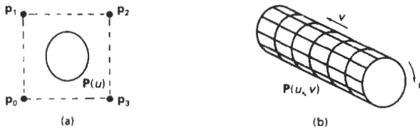
Figure 10-53 Constructing a solid with a translational sweep. Translating the control points of the periodic spline curve in (a) generates the solid shown in (b), whose surface can be described with point function P(u, v) .
